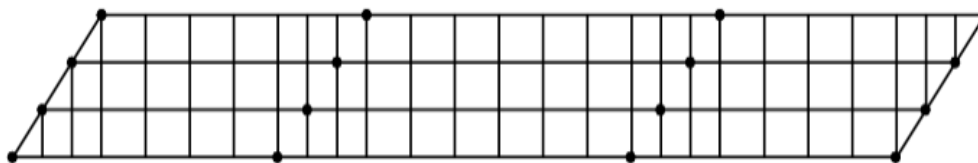
(c) Grillage for spans with large skew ( > 20^\circ )
